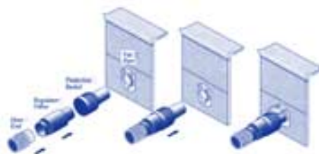
Figure 4: Use Protective Basket to prevent entrapment when the Regulator Valve is connected to a Dedicated Vacuum Port.
